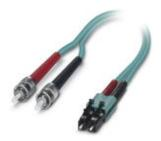
Assembled FO cable, zip cord cable, multi-mode fiberglass 50/125  $\mu$ m, OM3, plug: LC/B-FOC (ST), degree of protection: IP20, for installation in cable ducts or control cabinets, length: 2 m
