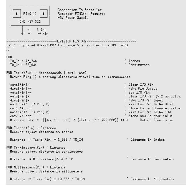
The ping.spin object is used in an example project with the Parallax 4 x 20 Serial LCD (#27979) to display distance measurements. The complete Project Archive can be downloaded from the Propeller Object Exchange at <a href="http://obex.parallax.com">http://obex.parallax.com</a>.
