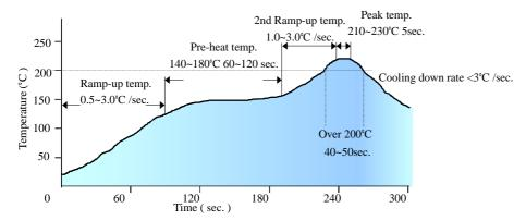
Note: The temperature refers to the pin of E48SC, measured on the pin +Vout joint.
