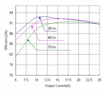
**igure 1:** Efficiency vs. load current for minimum, nominal, and maximum input voltage at  $25^{\circ}\text{C}$
