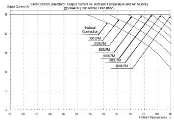
Figure 22: Output Current vs. ambient temperature and air velocity @ V<sub>in</sub>=48V(Transverse Orientation)
