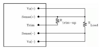
Figure 19: Circuit configuration for trim-up (increase output voltage)
