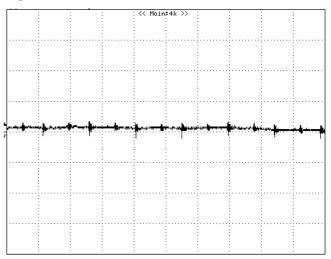
**Figure 11:** Input Terminal Ripple Current, i<sub>c</sub>, at full rated output current and nominal input voltage with 12µH source impedance and 33µF electrolytic capacitor (100 mA/div, 2us/div).
