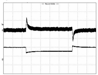
Figure 8: Output voltage response to step-change in load current (75%-50%-75% of lo, max; di/dt = 0.1A/μs). Load cap: 10μF, tantalum capacitor and 1μF ceramic capacitor. Top Trace: Vout (100mV/div, 200us/div), Bottom Trace: I out (5A/div). Scope measurement should be made using a BNC cable (length shorter than 20 inches). Position the load between 51 mm to 76 mm (2 inches to 3 inches) from the module..
