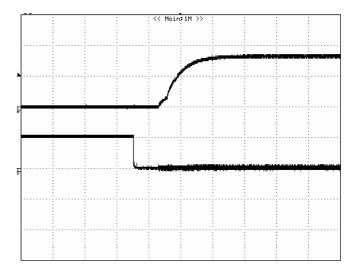
**Figure 4:** Turn-on transient at full rated load current (resistive load) (2 ms/div). Vin=48V.Top Trace: Vout, 2V/div; Bottom Trace: ON/OFF input, 5V/div
