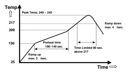
Note: The temperature refers to the pin of E48SC, measured on the pin +Vout joint.
