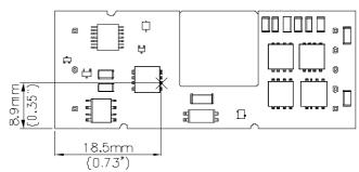
Figure 21: Hot spot temperature measured point.
