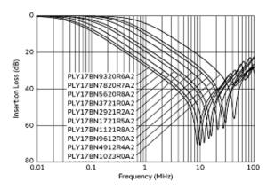
Common Mode Insertion Loss-Frequency Characteristics
