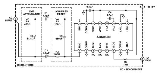
Figure 8. Circuit for Low Frequency Measurements
