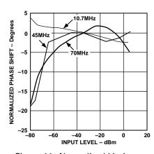
Figure 11. Normalized Limiter Phase Response vs. Input Level at 10.7 MHz, 45 MHz, and 70 MHz
