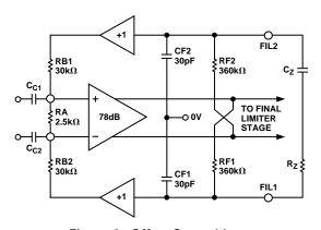
Figure 3. Offset Control Loop
