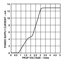
Figure 12. Supply Current vs. PRUP Voltage at +25°C
