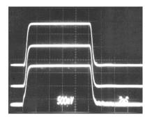
Figure 19.  $V_{LOG}$  Output for a Pulsed 10.7 MHz Input; Top Trace: –35 dBm to +5 dBm; Middle Trace: –15 dBm to –55 dBm; Bottom Trace: –35 dBm to –75 dBm
