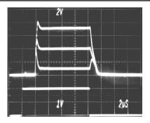
Figure 21. V<sub>LOG</sub> Output for 10.7 MHz CW Input with PRUP Toggled ON and OFF; Top Trace: +5 dBm Input; Middle Trace: -35 dBm Input; Bottom Trace: -75 dBm; PRUP Input from HP8112A: 0 to 4 V, 10 µs Pulsewidth with 10 kHz Repetition Rate
