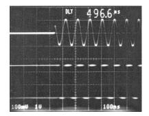
Figure 16. Limiter Response at Onset of 10.7 MHz Modulated Pulse at –75 dBm Using 200 pF Input Coupling Capacitors
