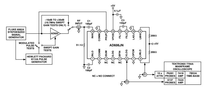
Figure 22. Test Setup for Characterization Data
