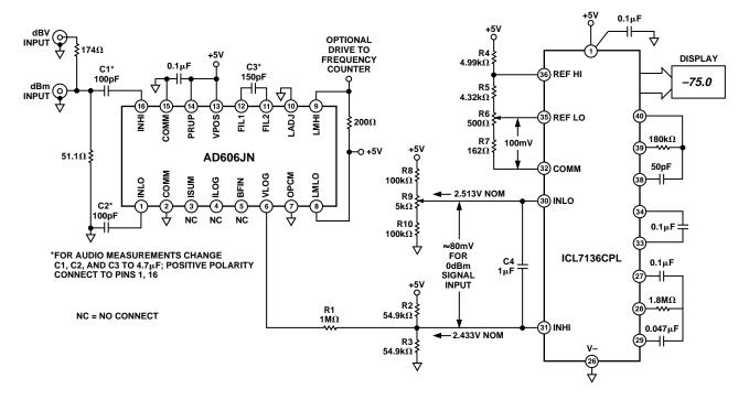
Figure 7. A Low Cost RF Power Meter
