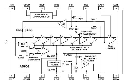
Figure 2. Simplified Block Diagram
