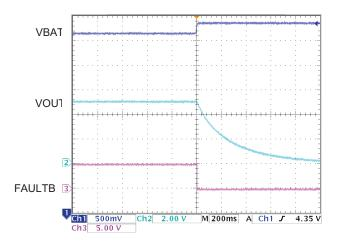
Figure 8. BAT-OVP, V<sub>VBAT</sub> Steps from 4.2V to 4.4V
