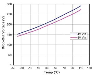
Figure 11. Drop-out Voltage vs. Temperature
