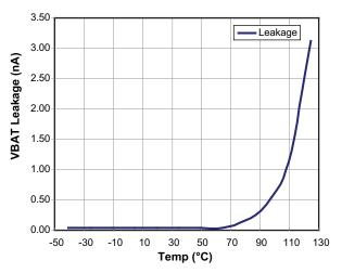
Figure 16. VBAT Leakage Current vs. Temperature
