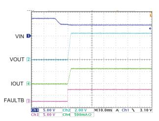
Figure 5. Recovery from OVP,  $V_{IN} = 7.5V$  to 5V
