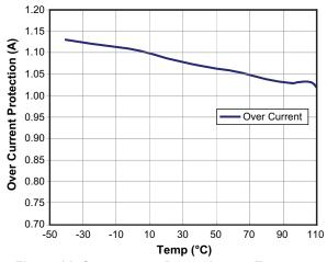
Figure 14. Over-current Protection vs. Temperature
