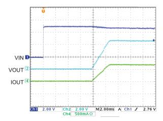
Figure 2. Normal Power-On Showing Soft-Start,  $R_{OUT}$  = 6.6 $\Omega$
