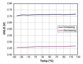
Figure 10. UVLO vs. Temperature
