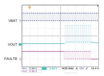
Figure 9. Battery OVP and Counter
