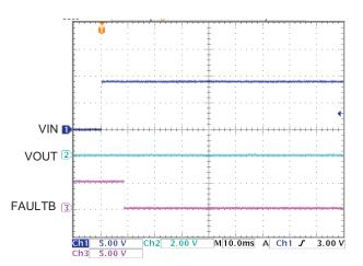
Figure 3. OVP at Power-On, V<sub>IN</sub> = 0V to 9V
