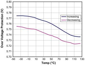
Figure 12. Over-voltage Protection vs. Temperature
