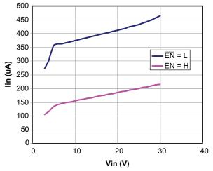
Figure 17. Supply Current vs. Input Voltage
