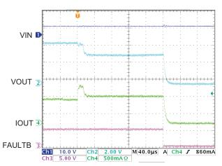
Figure 7. OCP,  $R_{OUT}$  Switches from 6.6 $\Omega$  to 3.3 $\Omega$ , Shows Current Limiting and Soft-stop
