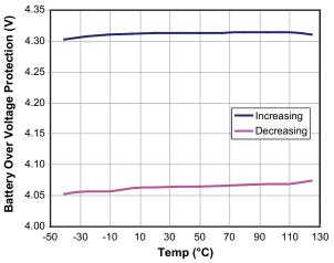
Figure 15. Battery Over Voltage Protection vs. Temperature
