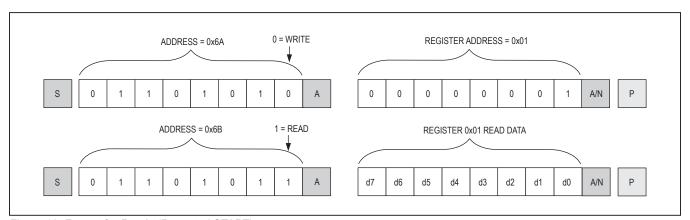
Figure 10. Format for Reads (Repeated START)
