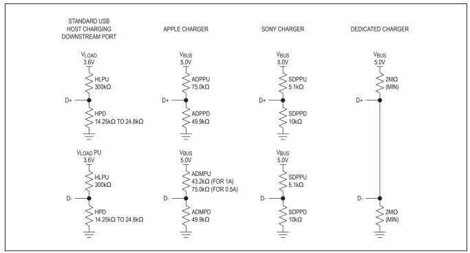
Figure 2. Standard USB Host Charging Downstream Port, Apple Charger, Sony Charger, and Dedicated Charger
