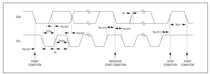
Figure 3. I<sup>2</sup>C Interface Timing
