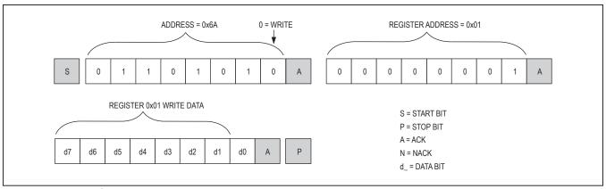
Figure 8. Format for I2C Write
