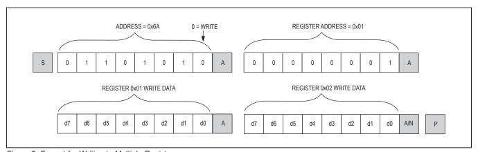
Figure 9. Format for Writing to Multiple Registers
