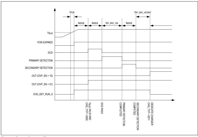
Figure 1. Charger Detection Timing
