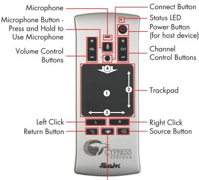
Button to switch between Motion Sensor and Trackpad
