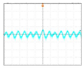
*Figure 8:* Output ripple & noise at 5Vin, 1.2V/12A out. (2us/div and 2mV/div)
