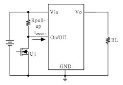
Figure 29: Positive remote On/Off implementation
