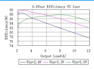
Figure 1: Converter efficiency vs. output current (0.6V out)
