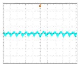
*Figure 7:* Output ripple & noise at 5Vin, 0.6V/12A out. (2us/div and 2mV/div)
