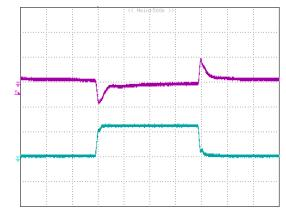
**Figure 22:** Typical transient response to step load change at 2.5A/µS from 0% to 50% to 0% of Io, max at 5Vin, 3.3Vout (100uS/div) (Cout = 47uF ceramic).top trace:Vout,0.2V/div;bottom trace:Iout:5A/div.
