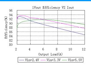
Figure 2: Converter efficiency vs. output current (1.0V out)
