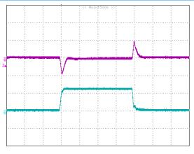
**Figure 19:** Typical transient response to step load change at 2.5A/µS from 0% to 50% to 0% of lo, max at 5Vin, 0.6Vout (100uS/div) (Cout = 47uF ceramic).top trace:Vout,0.2V/div;bottom trace:lout:5A/div.
