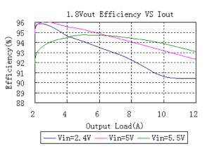
Figure 4: Converter efficiency vs. output current (1.8V out)
