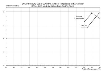
Figure 39: Output current vs. ambient temperature and air velocity@ Vin=3.3V, Vout=2.5V(Either Orientation)
