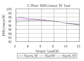
Figure 6: Converter efficiency vs. output current (3.3V out)
