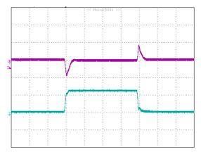
**Figure 21:** Typical transient response to step load change at 2.5A/µS from 0% to 50% to 0% of Io, max at 5Vin, 1.8Vout (100uS/div) (Cout = 47uF ceramic).top trace:Vout,0.2V/div;bottom trace:lout:5A/div.
