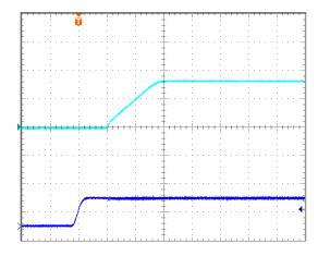
**Figure 18:** Turn on delay time at remote turn on with external capacitors (Co=800  $\mu$ F) 5Vin, 3.3V/12A out(2mS/div), Top trace:Vout 2V/div; bottom trace:Vin,5V/div
