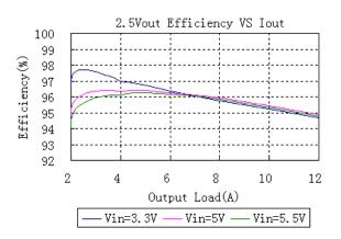
Figure 5: Converter efficiency vs. output current (2.5V out)
