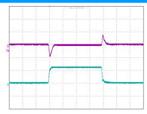
**Figure 20:** Typical transient response to step load change at  $2.5A/\mu S$  from 0% to 50% to 0% of lo, max at 5Vin, 1.2Vout (100uS/div) (Cout = 47uF ceramic).top trace:Vout,0.2V/div;bottom trace:lout:5A/div.
