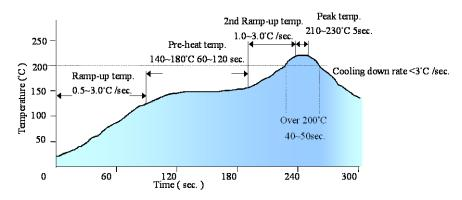
Note: The temperature refers to the pin of DCM, measured on the pin Vout joint.
