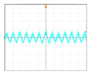
**Figure 10:** Output ripple & noise at 5Vin, 3.3V/12A out. (2us/div and 2mV/div)
