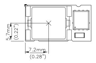
Figure 37: Temperature measurement location The allowed maximum hot spot temperature is defined at 107  ${\mathcal C}$
