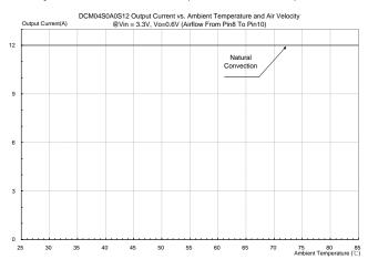
Figure 42: Output current vs. ambient temperature and air velocity @Vin=3.3V, Vout=0.6V(Either Orientation)
