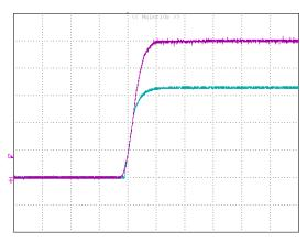
**Figure 24:**Tracking at 5Vin, 3.3V/0A out(1mS/div), tracking voltage=5V,top trace:Vseq,1V/div;bottom trace:Vout,1V/div
