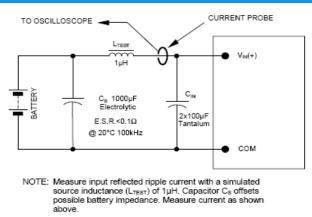
Figure 25: Input reflected-ripple test setup
