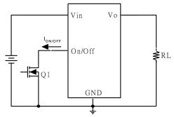
Figure 28: Negaitive remote On/Off implementation
