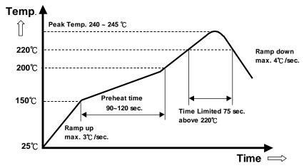
Note: The temperature refers to the pin of DCM, measured on the pin Vout joint.
