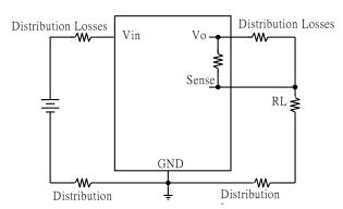
Figure 30: Effective circuit configuration for remote sense operation
