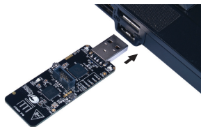
Fig-2: Powering the CySmart USB Dongle
